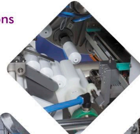
TUBE LOADING STATION 1
